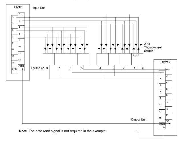
The following example illustrates connections for an A7B Thumbwheel Switch.
